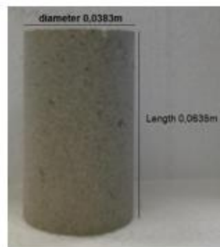
Figure 3. Core sample - sandstone Berea Buff
