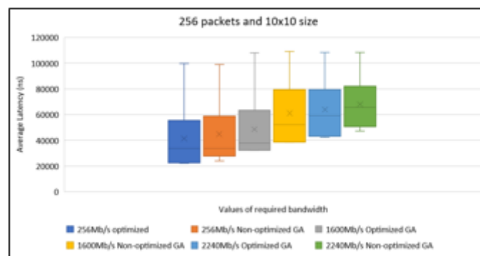
Figure 5: Three variations of the application, keeping the same number of packets and size, but varying the required bandwidth.
