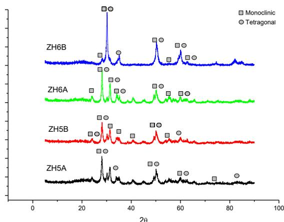
Figure 02: X-ray diffraction of zirconium oxide synthesized by homogeneous precipitation reaction.
