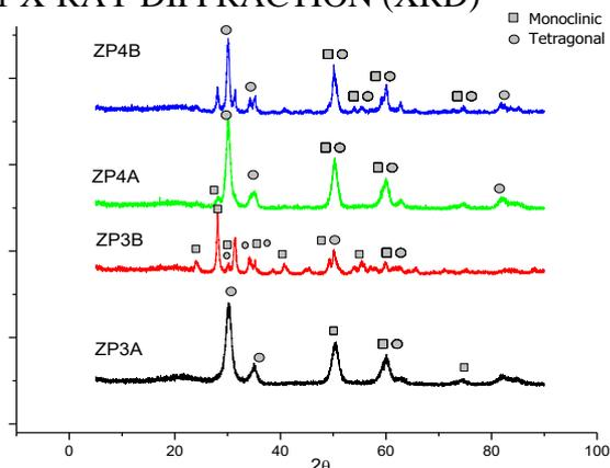
Figure 01: X-ray diffraction of zirconium oxide synthesized by Pechini method
