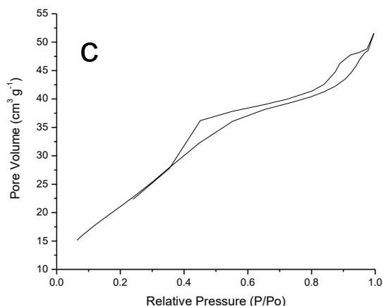
Figure 05 : Adsorption/desorption Isotherms for samples (A) Pechini with ethylene glycol, (B) Pechini with glycerol, (C) homogeneous precipitation with urea.
