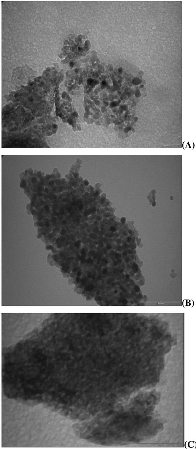
Figure 06: Micrograph of samples of the Pechini ZP3A (A), ZP4A(B) and homogenous precipitation respectively ZH5A(C).
