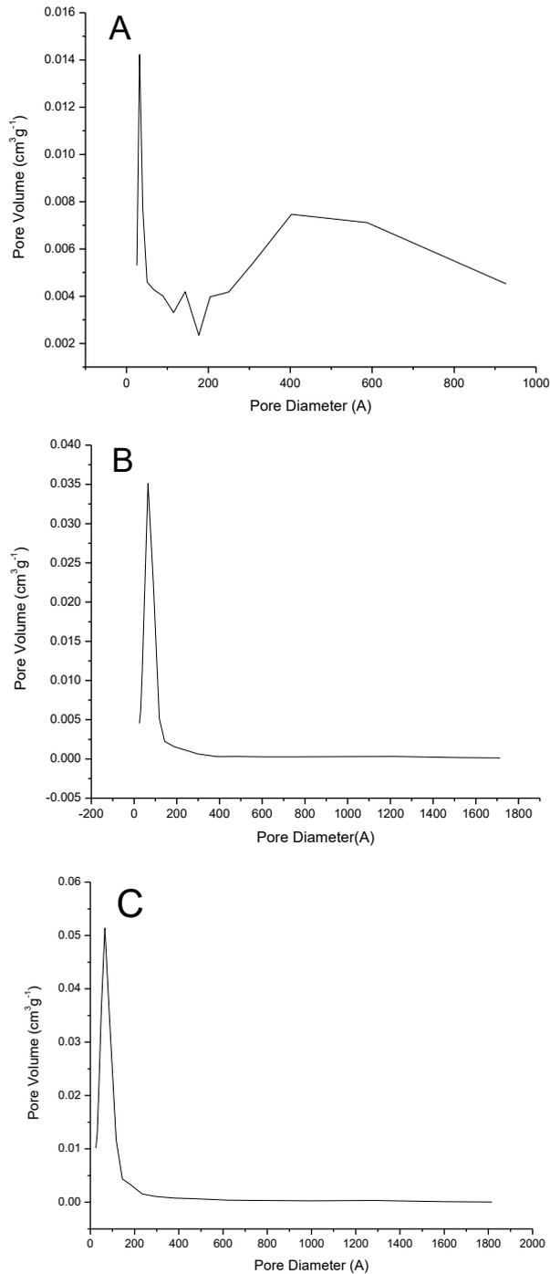
Figure 04: Distribution of pore volume for samples (A) Pechini with ethylene glycol, (B) Pechini with glycerol, (C) homogeneous precipitation with urea.
