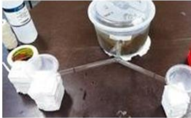
Fig 4 – Set up a scheme for the food selection experiment where a treatment option was placed in each pot at the end of the Y-tube.
