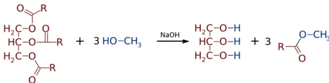
Figure 1: Transesterification reaction in alkaline mean.
