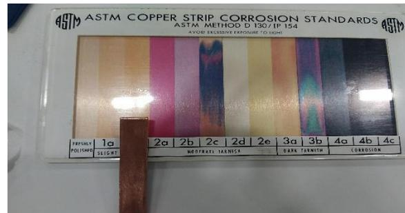
Figure 8: Corrosion check on copper blade.
