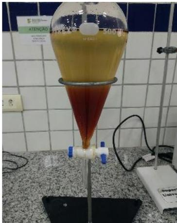
Figure 2: Separation of phases. Biodiesel on the top and glycerin on the bottom.
