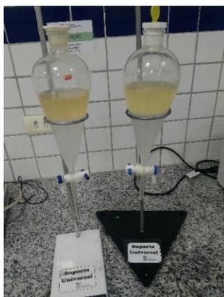
Figure 3: Washing procedure to remove KOH.
