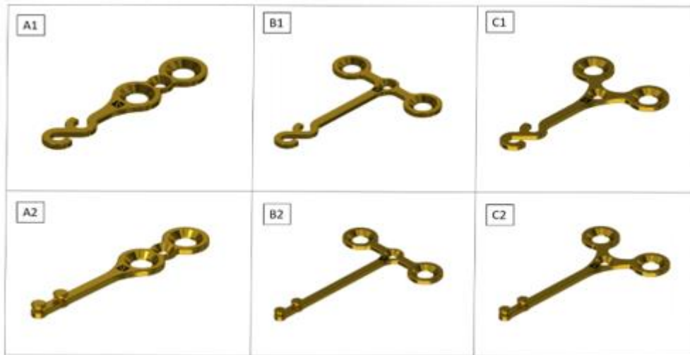
Figure 1. Three-dimensional models of the studied miniplates separated by types. A1: 20 mm, A2: 23 mm, B1: 20 mm, B2: 19 mm, C1: 19 mm, C2: 23 mm.
